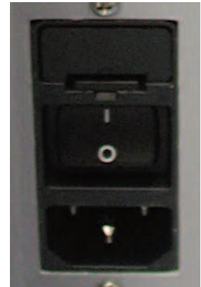
Figure 5-2. Power Switch I = ON, O = Off
