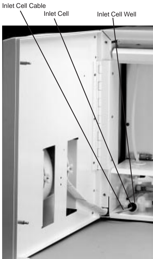
Figure 8 Inlet Cell Installation and Location
