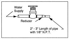
Figure 3 Shut-off Valve
